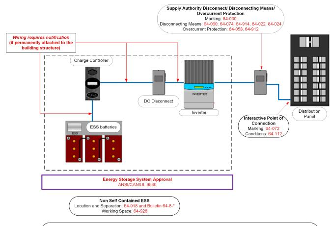
Note: For other than self contained ESS, the approval of an assembled ESS shall include all equipment forming the system. As a minimum, a battery ESS shall include a charge controller and storage batteries.
