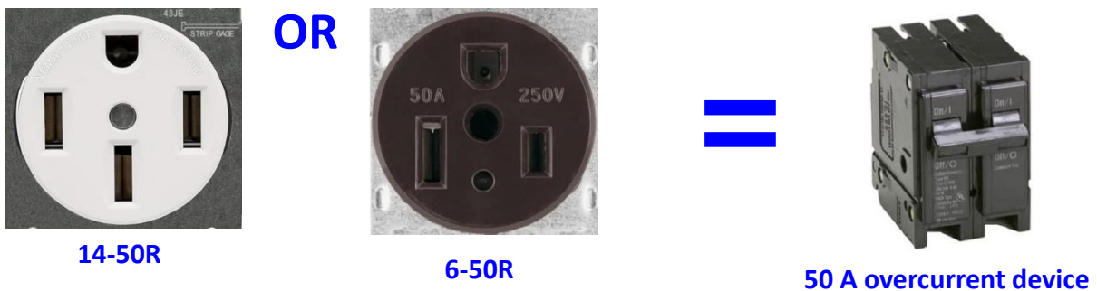
Diagram B5 – 50 A receptacle with 50 A overcurrent device
